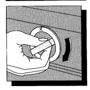
Press and turn the programme dial **clockwise** until letter **K** on the dial coincides with the red marker line.
